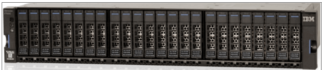
Figure 1-7 IBM Storwize V7000 Generation 3 (2076-724)
