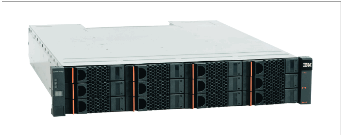
Figure 1-10 IBM FlashSystem 5015 and 5035 LFF control enclosure front view
