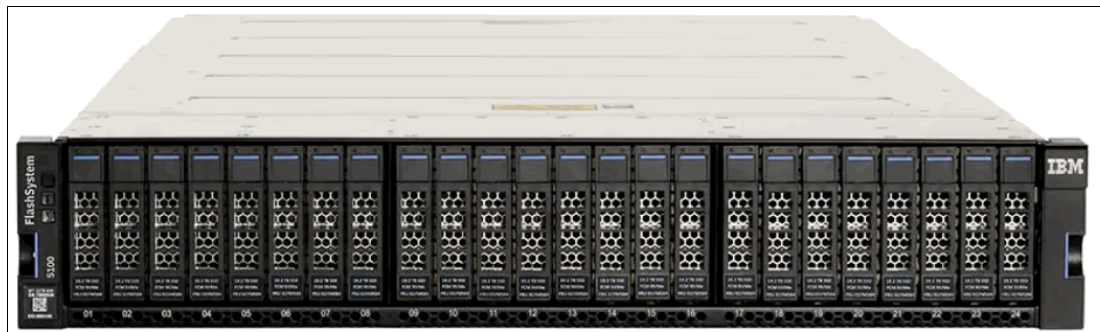
Figure 1-11 IBM FlashSystem 5100 front view showing the 24 NVMe drives installed
